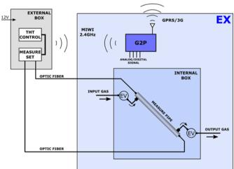
The internal box is installed within the classified area, it contains the measuring tube, the solenoid valves and the gas filtering and pressure reduction sections.
