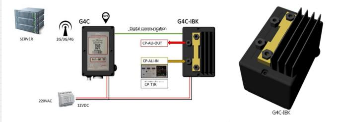
The **G4C-IBK** is an accessory of the G4C remote monitoring device that allows synchronized current interruption to perform on/ off surveys. With an integrated solid state relay, the unit allows interruptions to be carried out with very high frequency to perform DCVG, CIPS or routine on/off surveys.
