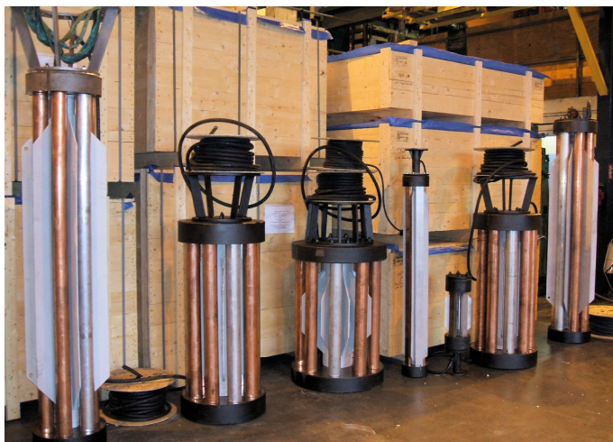
Typical examples of pump mounted Cuprion™ Anti Fouling Electrodes
