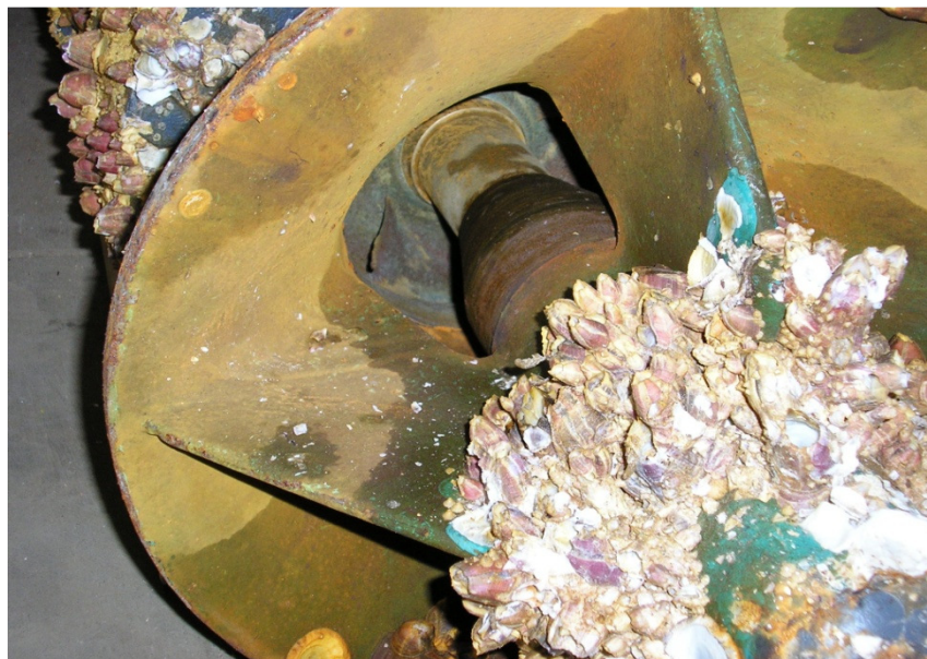
Picture shows typical example of hard fouling
